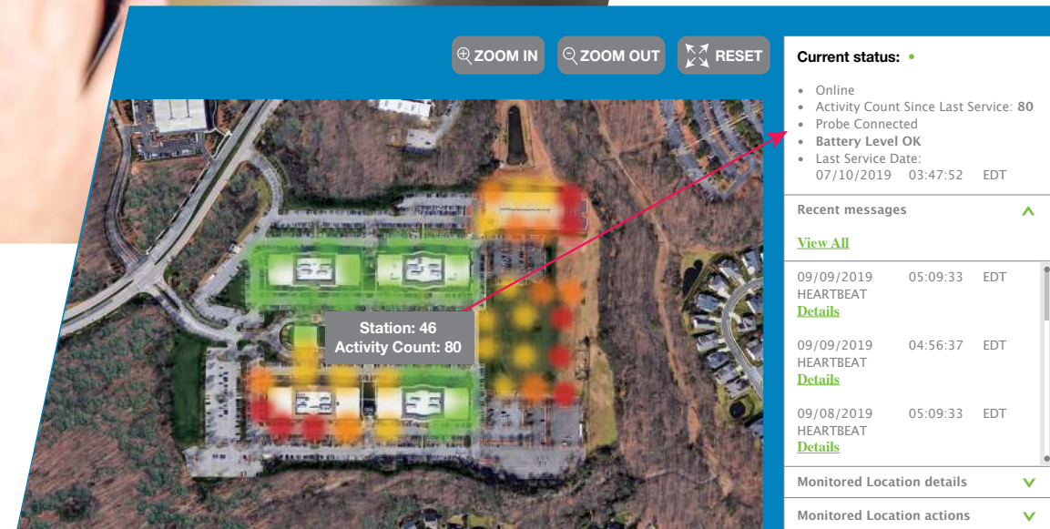
Heat maps showing areas of rodent pressure are automatically generated by capture data provided from the network of deployed devices.
