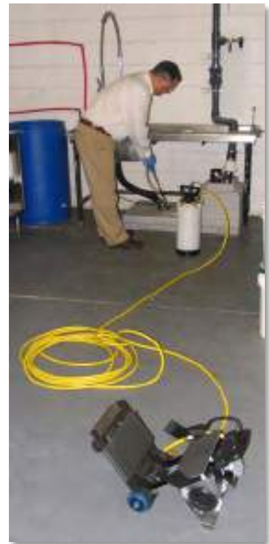
The optional Air Line 50' extension hose allows technicians to separate the tank from the utility cart while still accessing the electric compressor.
