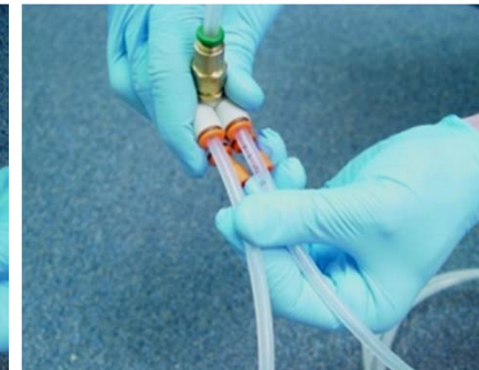
Additional 4 line manifold(s) are connected
