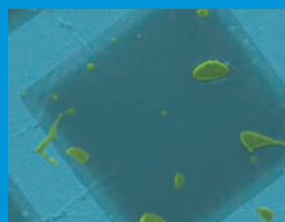
LambdaStar™ Insecticide capsule fully collapses under heat and pressure.
