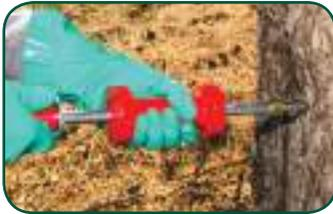
**It is important** to keep the rear handle of the Tip Setter directly behind the tip in order to guide the tip into the tree without bending the tip. When inserting or removing Portle or Palm Tips, it is important to keep the setter perpendicular to the tree. Do not twist or move the setter or injector unit side to side, as this may bend or break the injection tip.
