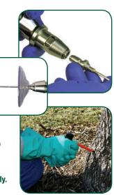
**Insert a WedgeChek** into the site where bark core has been removed. Place the WedgeChek (#72) on the protruding pin on the handle of the WedgeChek Punch, then insert the WedgeChek directly into the punched site until the WedgeChek flange is flush with the outer bark of the tree. The barbs on the WedgeChek will secure it in the bark. See notes below on treating thinbarked trees.
